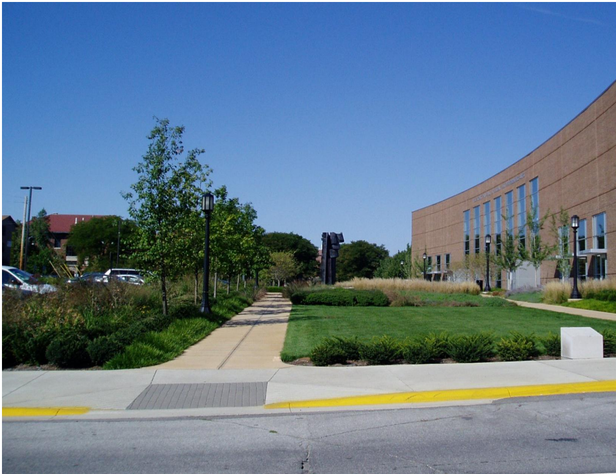
A Bioswale (left) Collects Parking Lot Runoff Near Pao Hall of Visual and Performing Arts
